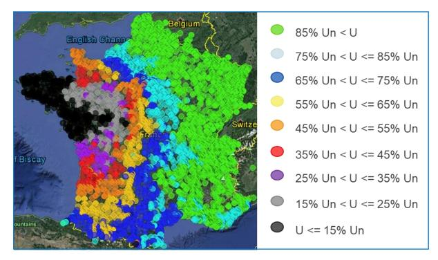
Figure 6. Example of propagation of the fault in the 400kV western part of the French transmission system
