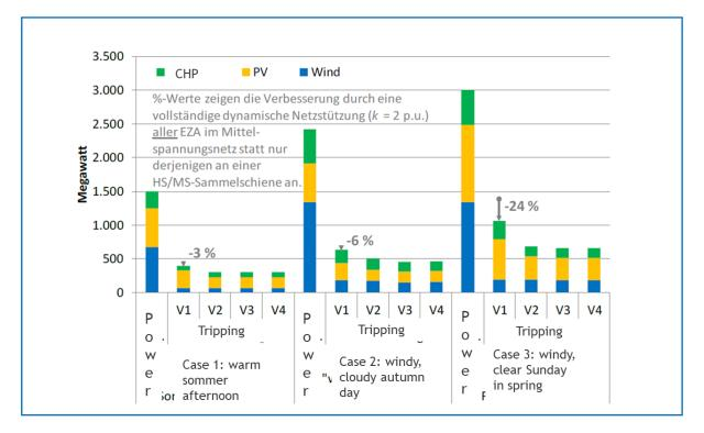
Figure 9. Dynamic grid support: V1: no, v2 limited, v3 full, v4: full plus active power. %-values: improvement of full dynamic grid support for whole distribution generation at MV network (not only the bus bar connected)
