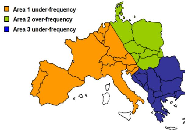
System split is identified as a grid extreme contingency leading to separation of the system into asynchronous zones.
