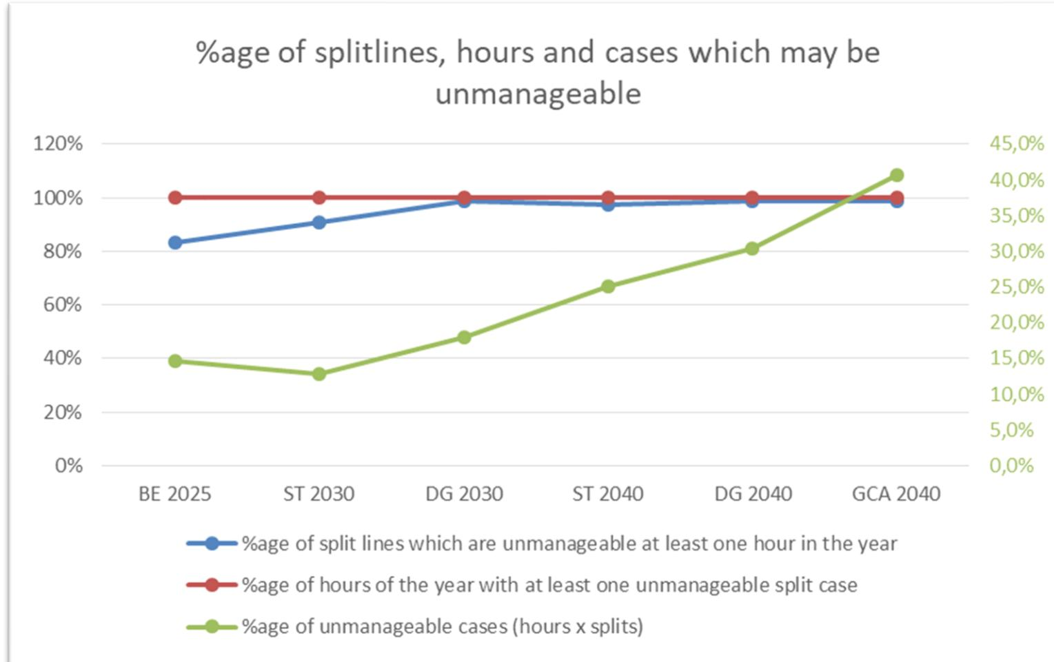
**The red line** at 100% shows that at any hour of the year at least one split can be unmanageable (RoCoF higher than 1Hz/s)
