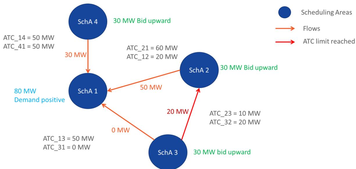
Figure 7: Example of a feasible flow solution
