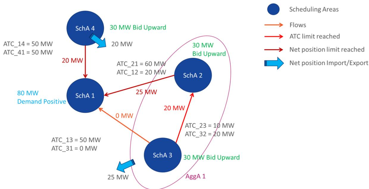
Figure 12: Feasible flow solution with net position limit
