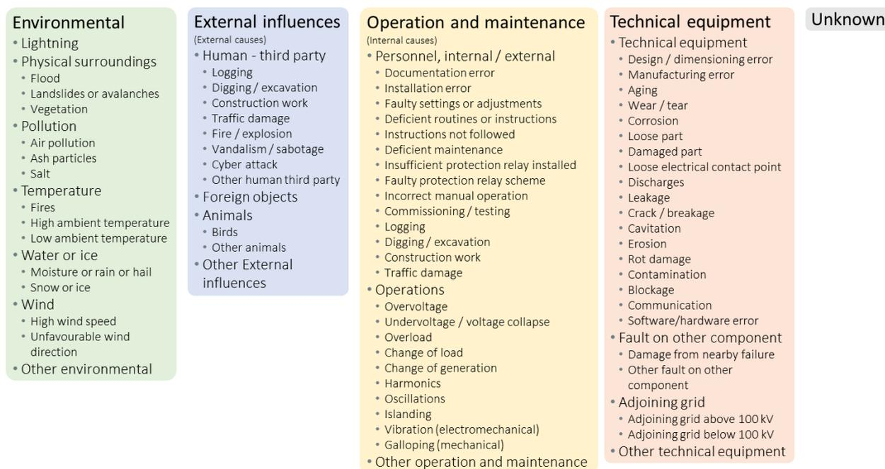
Figure 6.1 The cause scheme with 5 top-level categories: environmental causes, external influences, operation and maintenance, technical equipment, and unknown. The top-level categories have sub- and sub-subcategories to further detail the nature of the causes. The cause scheme does not indicate the significance or the magnitude of potential consequences of a specific cause. It is only used to categorise causes or threats, which may be seen in the power system by a European TSO, by their nature.
