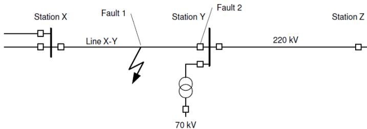
Figure 0.4 Line fault with a circuit breaker malfunction
