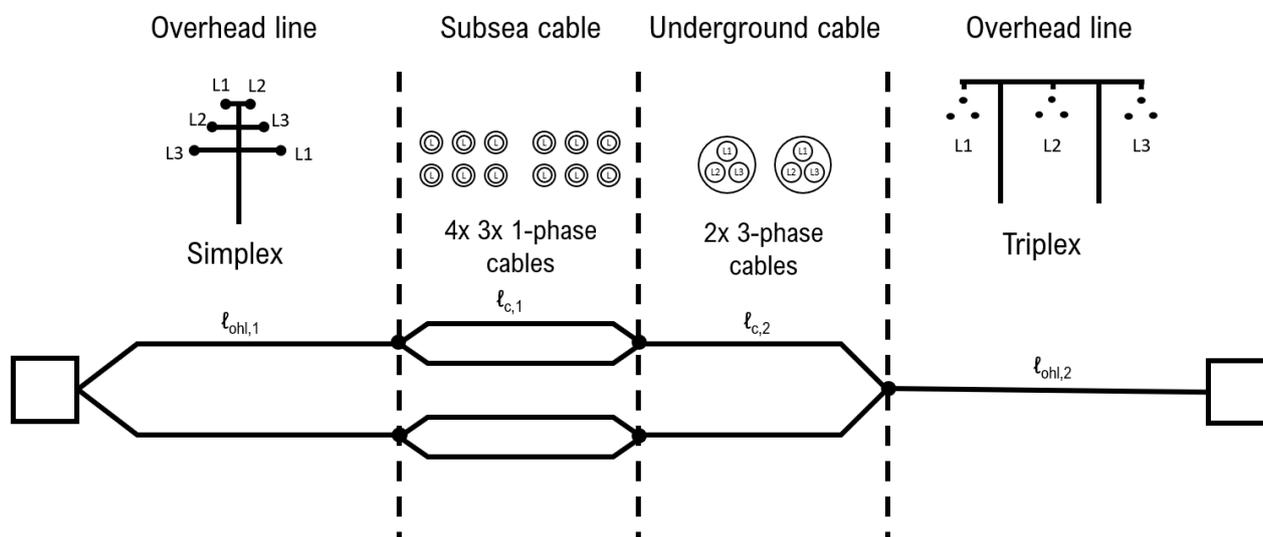
Figure 7.3 Circuit length and physical length calculation example of an HVAC overhead line and subsea/underground cable section. The diagram is a 3-phase single line. Circuit length only considers a single conductor length, ignoring parallel lines and cables, between the circuit breakers. Physical length for the overhead line sections multiplies the circuit length by the number of 3-phase sets, and physical length for the cable sections multiply circuit length by the number of physical cables.
