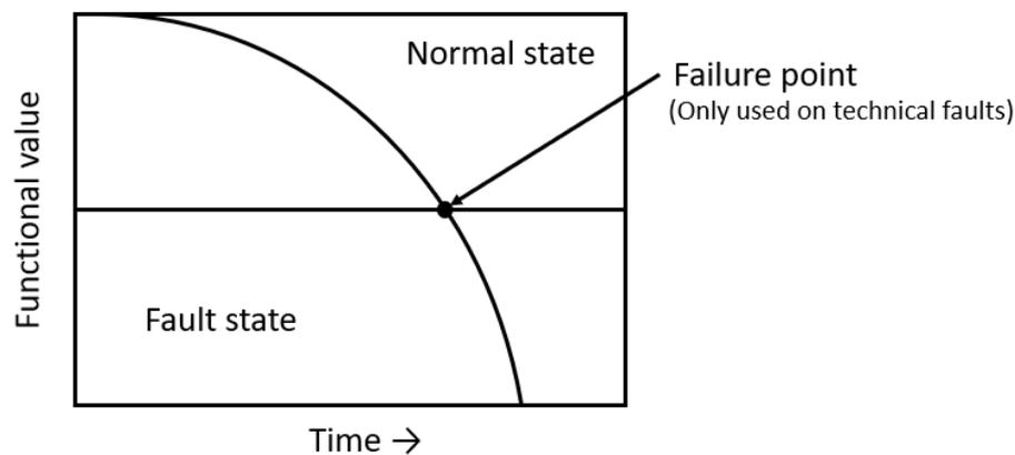
Figure 4.1 Failure point of an item occurs when the item’s state transitions from normal state to fault state. A technical fault is defined in Section 4.9.8.
