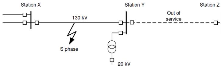
Figure 0.20 Line fault with an end-user outage in the downstream network.
