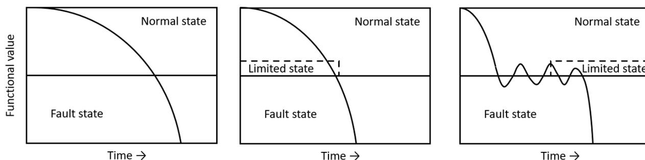
Figure 4.2 Transitioning from normal state or limited state to faults state is normally called a fault. If transition between states is intermittent, it is an intermittent fault.
