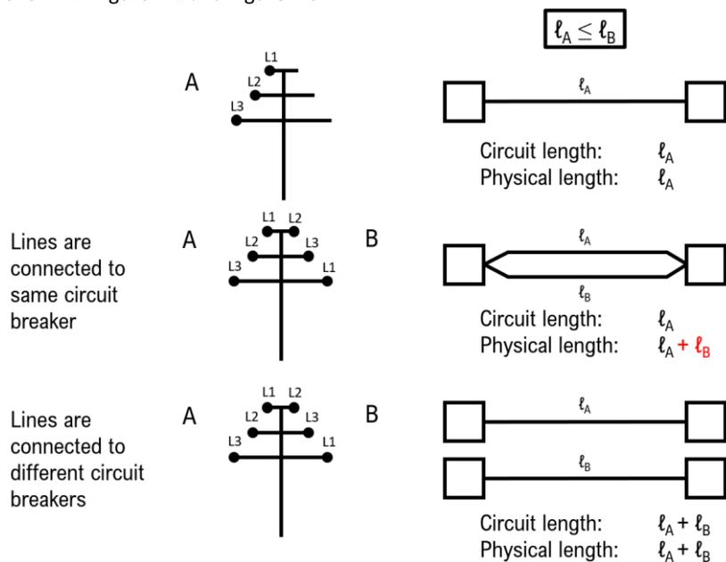
Figure 7.1 How to calculate circuit length and physical length for different HVAC overhead line configurations. Circuit length is defined as the shortest conductor path between two circuit breakers. Physical length is defined as the circuit length multiplied with the number of installed 3-phase sets.
