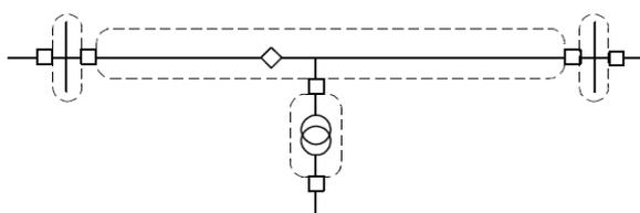
Figure 4.11 A system unit is delimited by circuit breakers as indicated by the dotted lines. Disconnectors do not delimit system units. This system unit must be defined as being of the line type.
