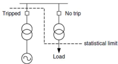
Figure 0.9 Fault in a generator connected directly to the transmission network
