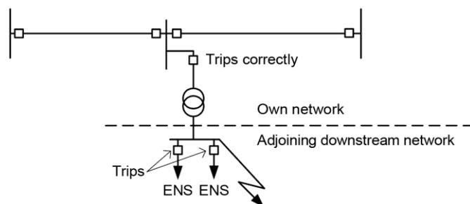
Figure 4.7 A failure in the downstream network causes an outage in a system unit within the statistical area resulting in ENS. As an outage causing ENS also occurs within the statistical area, this ENS must be included in the statistics with the fault sub-cause 'Adjoining grid below 100 kV'.
