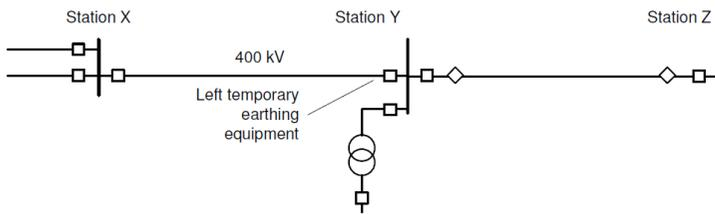
Figure 0.7 Line disconnection caused by temporary earthing equipment being left on the X-Y line in station Y.
