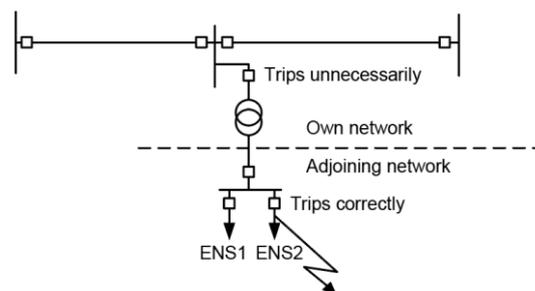
Figure 4.8 This scenario includes a breaker on the lower side of the transformer, in this case a breaker within the statistics trips unnecessarily. The ENS values should be separated if possible. The first ENS (ENS2) is for the line where the feeder tripped correctly (fault in another statistical area) and the other ENS (ENS1) is for the feeder where the breaker tripped unnecessarily.
