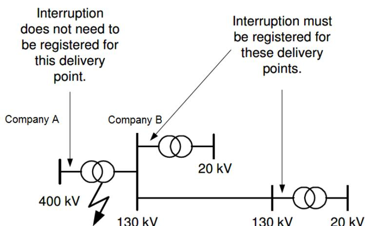
Figure 4.3 It is only the delivery points from the transmission network to low voltages that are registered
