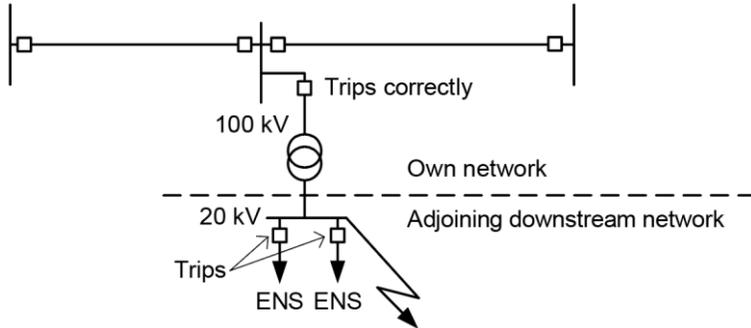
Figure 0.23 Fault on the lower side of a 100/20 kV transformer
