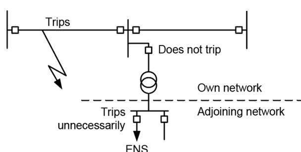
Figure 4.10 Incorrect settings in the protection system causes faults in the downstream network. The resulting ENS should not be registered because no system unit, that is transmitting to the downstream network, is affected by the outage.
