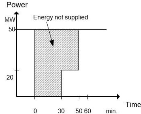
Figure 0.21 A visual representation of how to calculate the energy not supplied in the example of Section 0.
