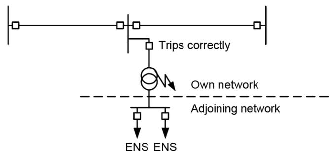
Figure 4.9 ENS must be recorded when the transformer is affected by a fault that causes an outage.
