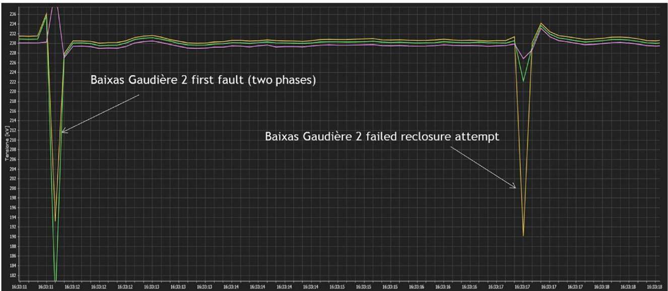
Figure 27: PMU recording of voltages in Baixas (20 ms sampling rate).
