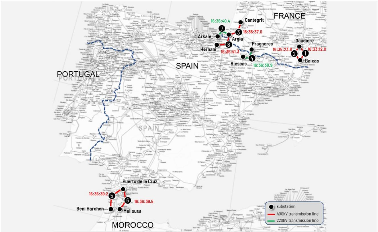
Figure 10: Geographical location of main tripped transmission system elements.
