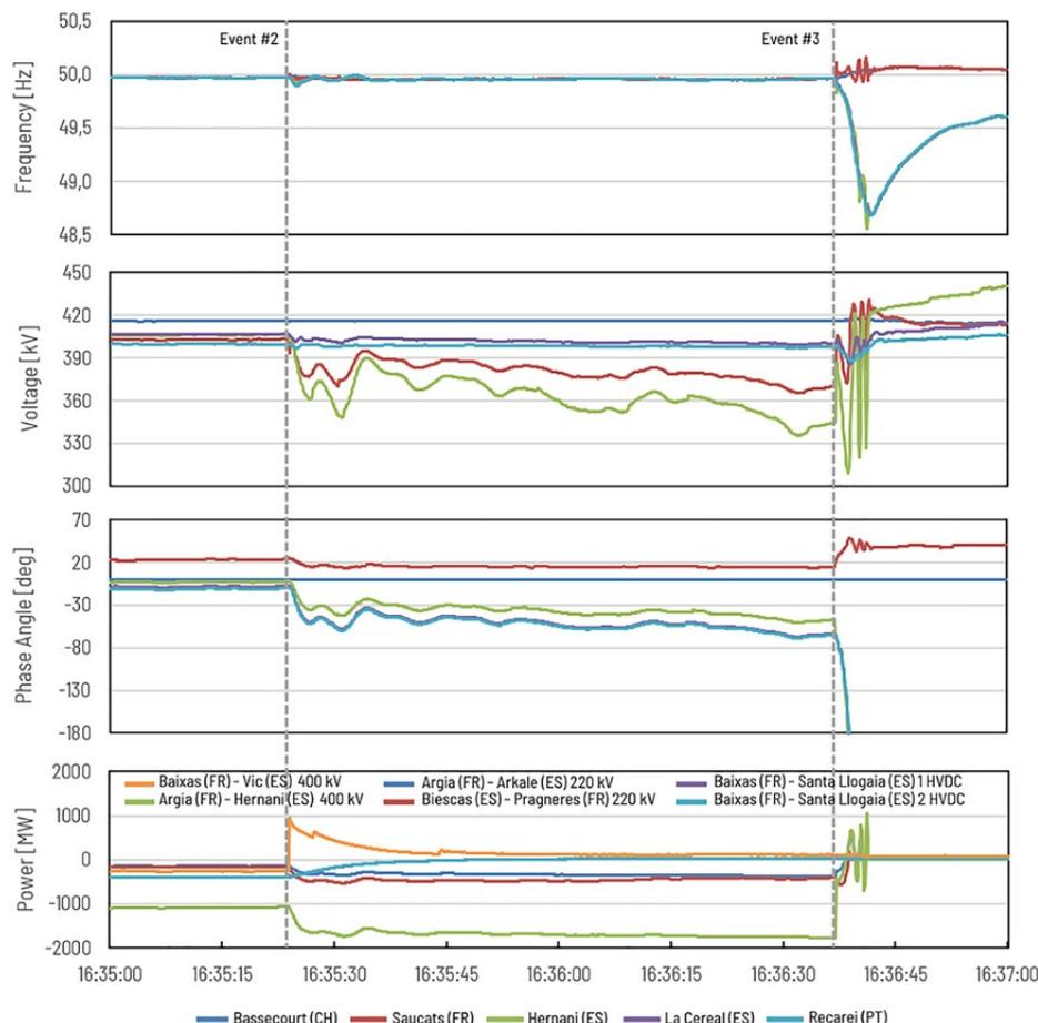
Figure 12: Frequencies, voltages, voltage phase angle difference and active power of France-Spain tie lines as measured by PMUs (reference for voltage phase angle difference is Bassecourt (CH) substations).
