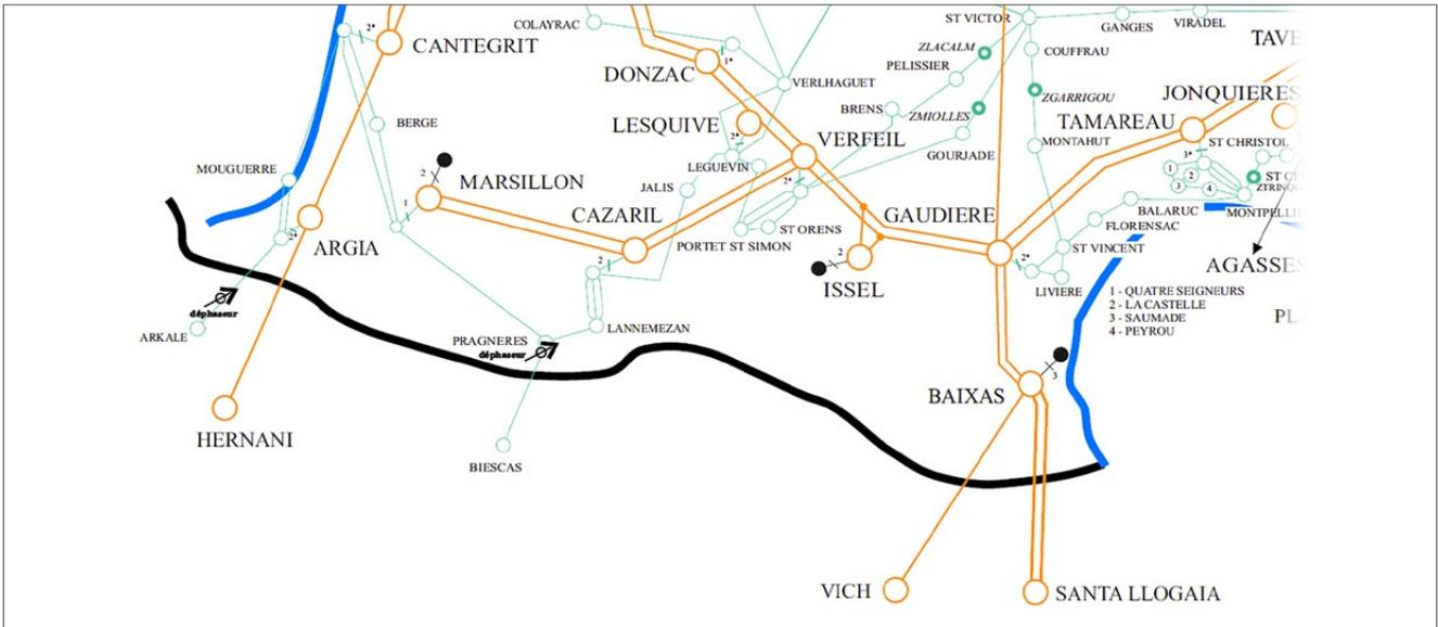
Figure 4: Grid map of the South of France (400 kV in orange; 225 kV in green).
