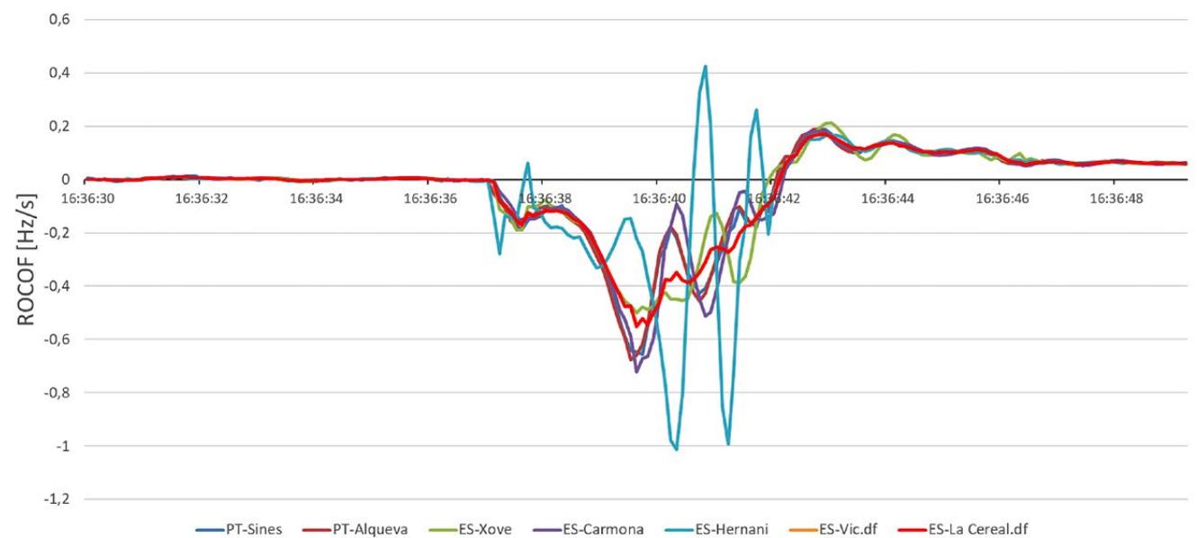
Figure 16: ROCOF measured in several substations on the Iberian Peninsula.
