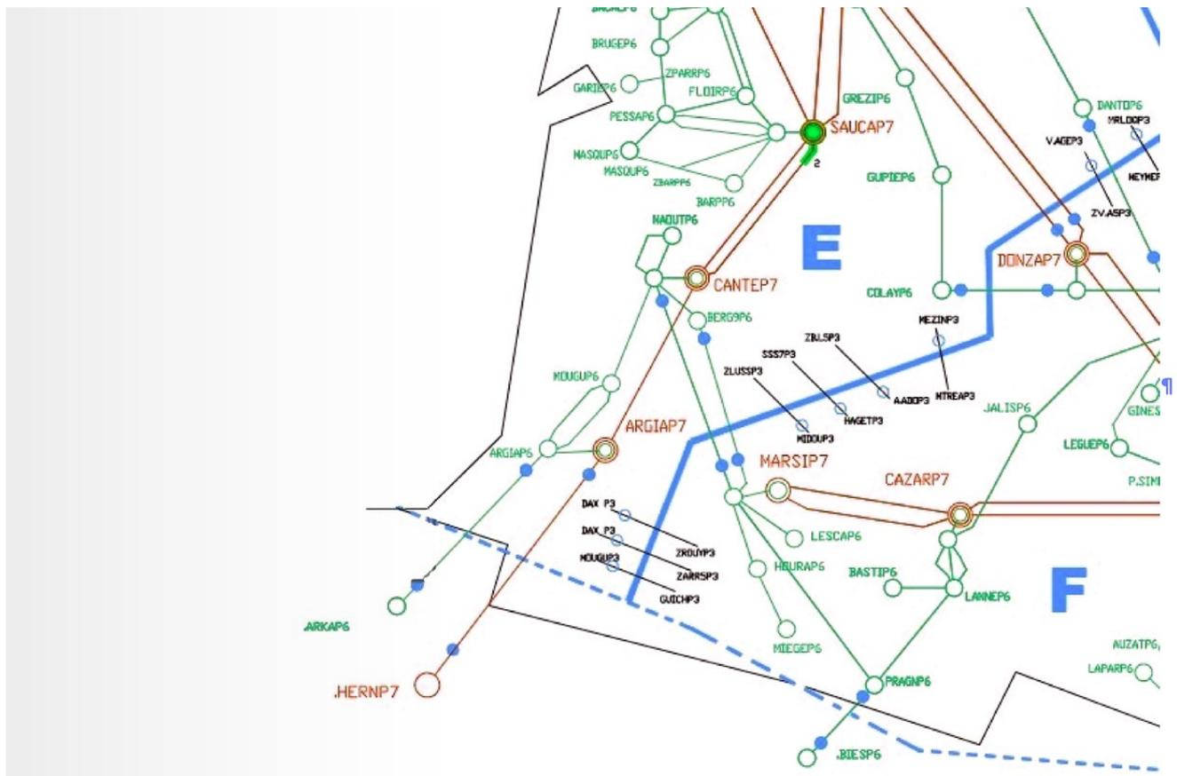
Figure 37: "E" DRS area, with connection lines with "F" area. Red lines: 400 kV, Green lines: 225 kV, Black lines: 63 kV
