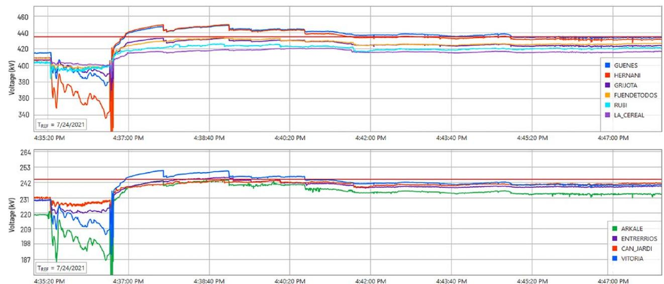
Figure 19: Voltages measured by PMUs at 400 kV and 220 kV transmission networks.
