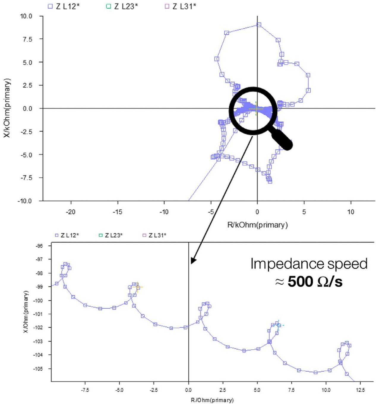
Figure 39: impedance trajectory seen by protection.
