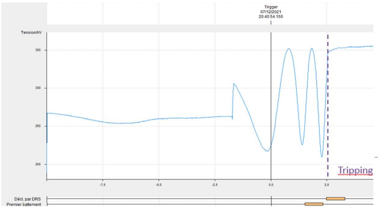
Figure 38: Voltage beats at Argia 400 kV substation (device not time synchronised).
