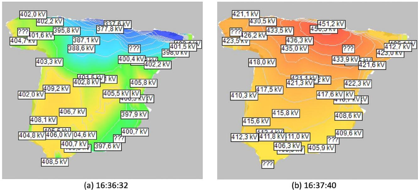
Figure 18: Voltages in Spanish 400 kV network.
