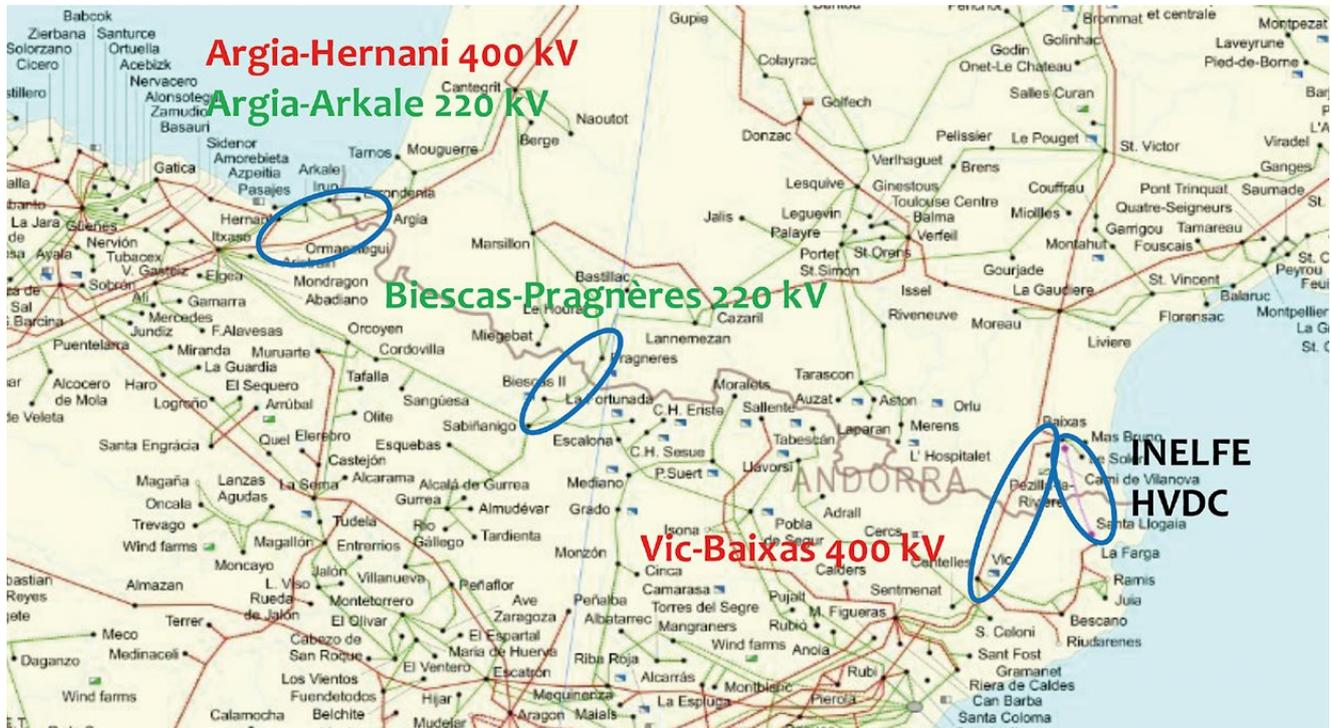
Figure 20: Transmission network in the French-Spanish border.
