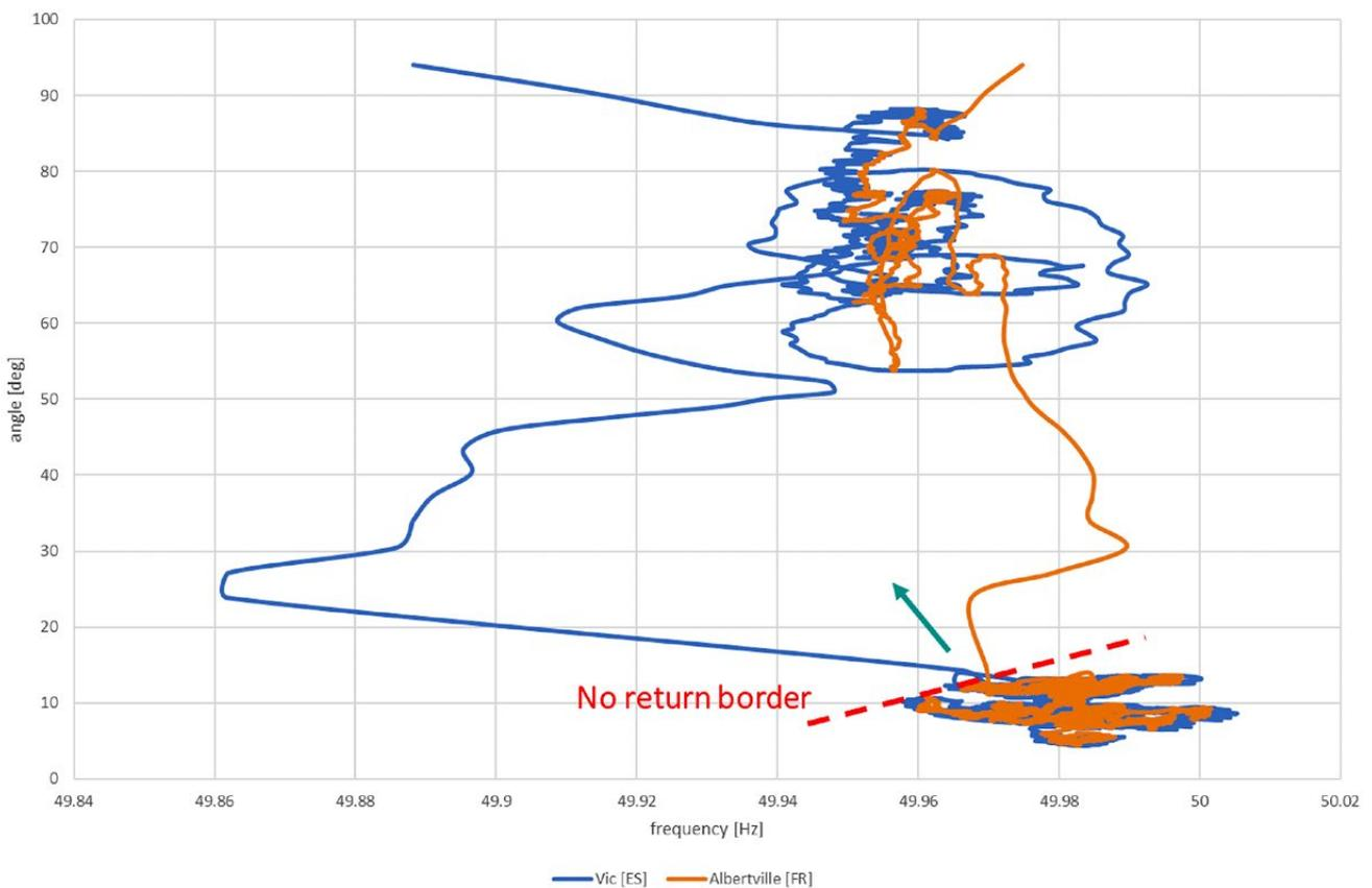
Figure 17: Phase plan (angle difference, frequencies) measured in France and Spain.
