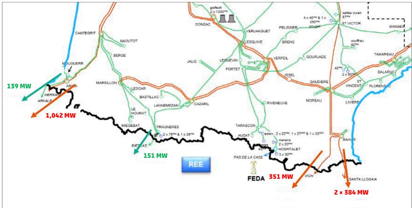
Figure 7: Simplified view (225 kV in green, 400 kV in red) of the south-west French transmission system and the exchanges with Spain before the event.
