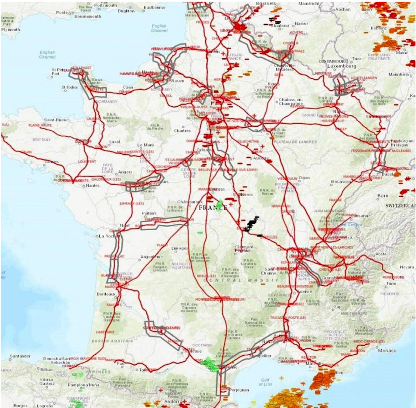
Figure 43: Real-time monitoring of lightning events close to the 400 kV French Grid.
