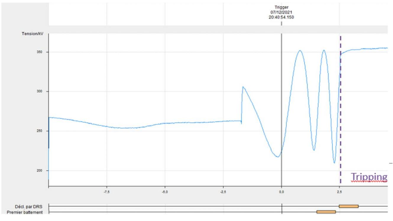
Figure 38: Voltage beats at Argia 400 kV substation (device not time synchronised).
