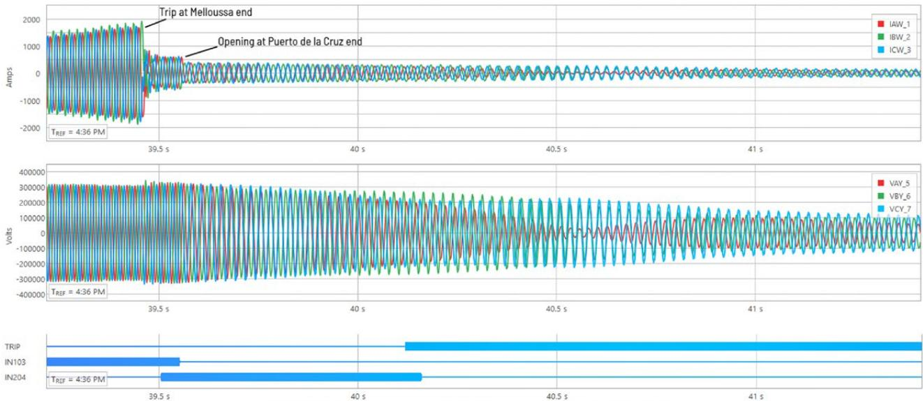
Figure 33: Melloussa bay at Puerto de la Cruz 400 kV substation relay recording (IN103: breaker position, IN204: direct transfer trip reception).
