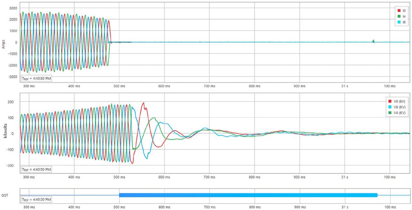
Figure 35: Arkale 220 kV bay Argia DFR recording (device not time synchronised).
