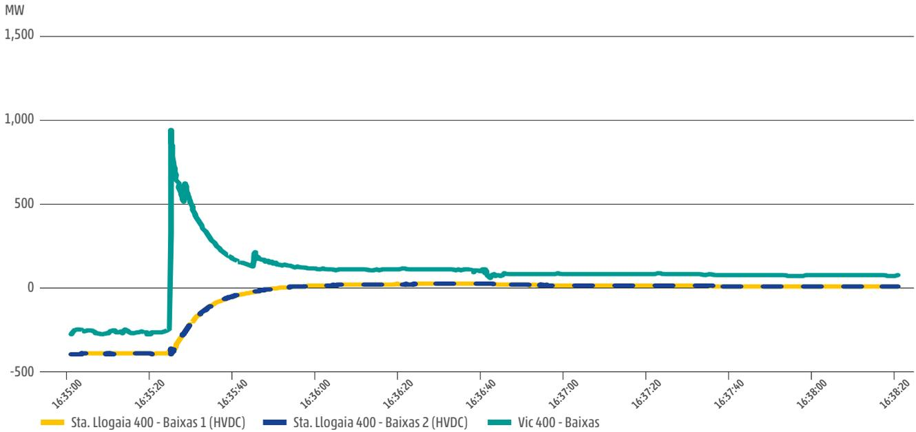
Figure 22: Active power of eastern France-Spain tie lines (positive means power transfer from Spain to France).
