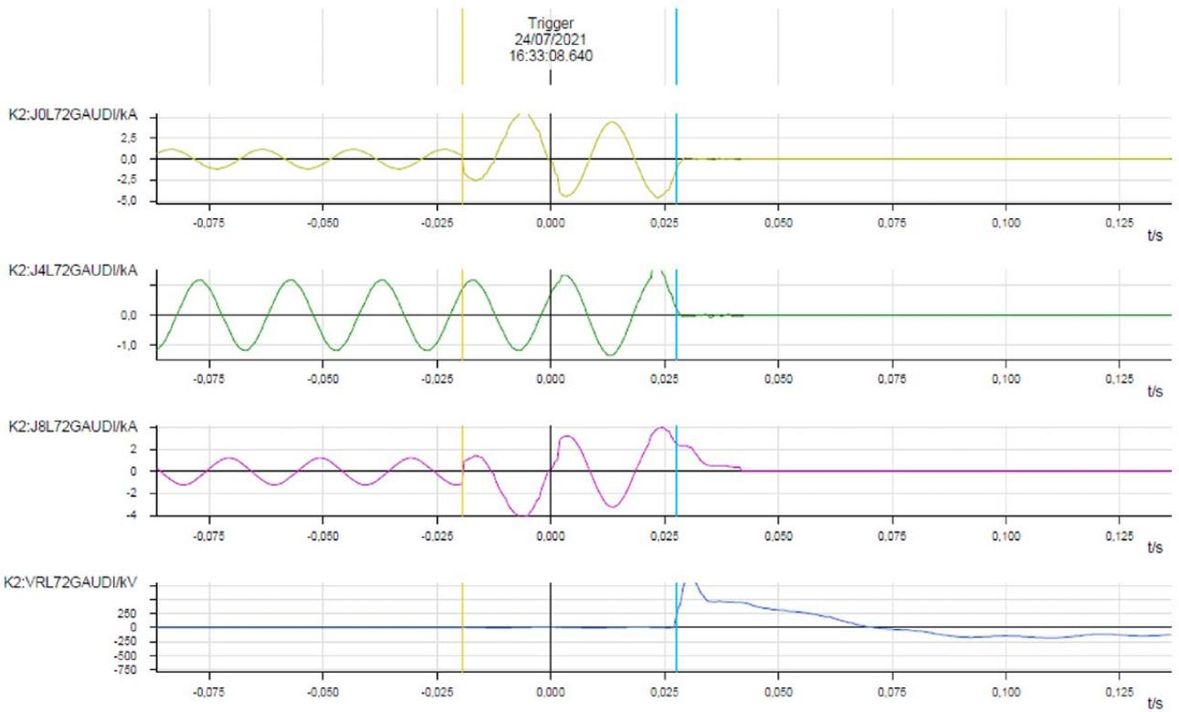
Figure 25: Oscillography recording of currents of Gaudière bay.
