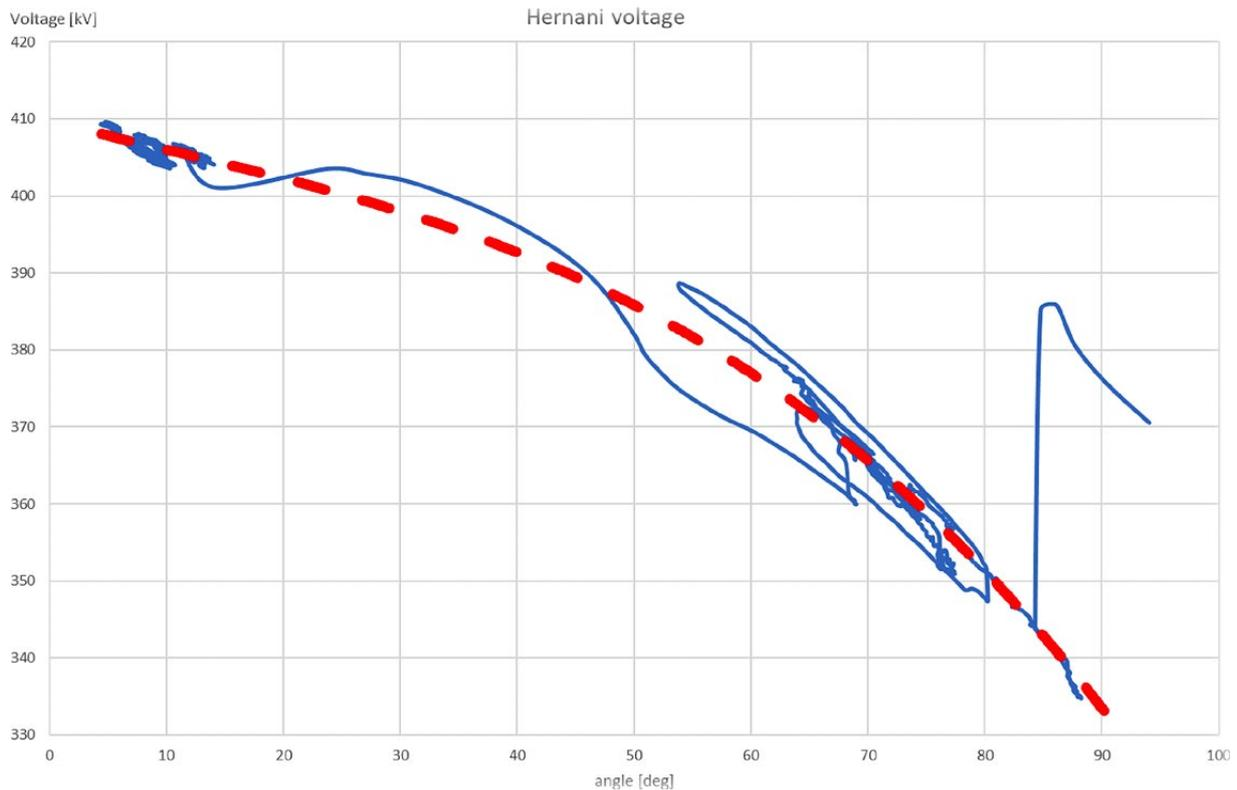
Figure 13: Voltage magnitude versus phase angle difference in Hernani substation - PMU recording (phase angle referred to Bassecourt (CH)).
