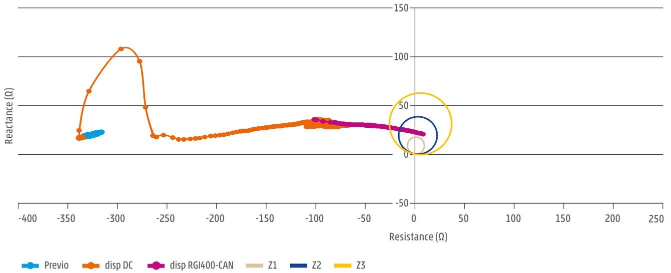
Figure 31: Pragneres bay at Biescas 220 kV substation: Impedance evolution using PMU data.
