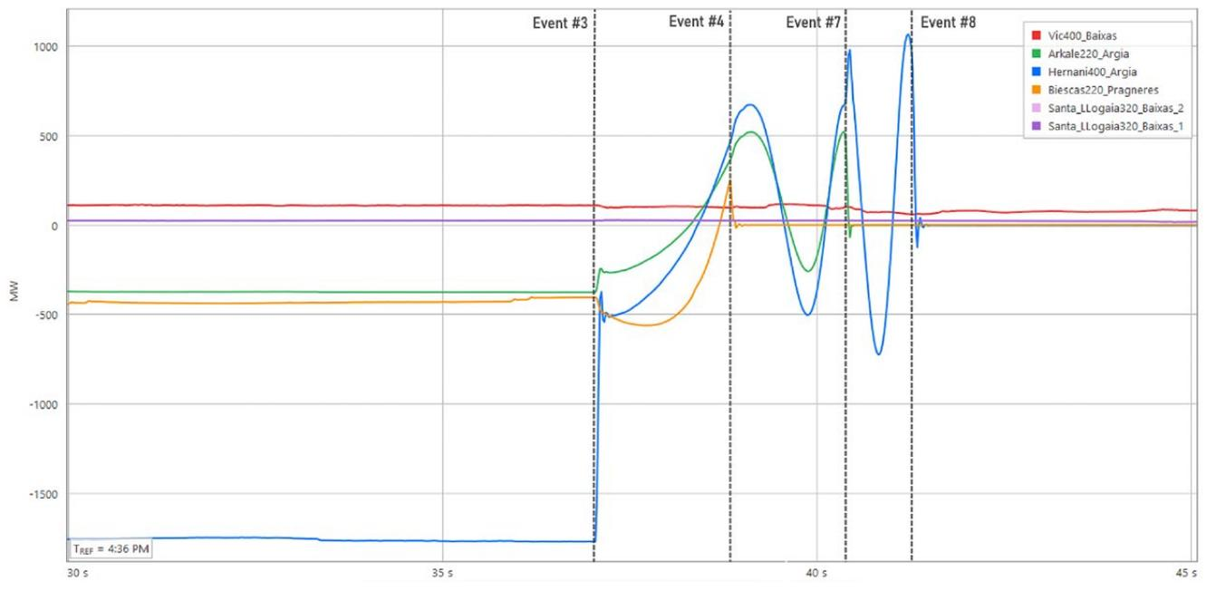
Figure 15: Active power of France-Spain tie lines as measured by PMUs (positive indicates power transfer from Spain to France).
