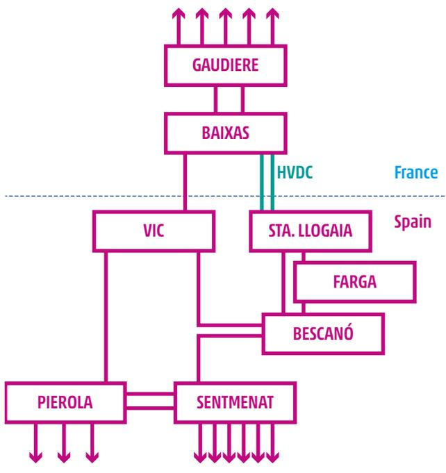
Figure 21: AC-DC corridor formed by the HVDC link and the Vic-Baixas line
