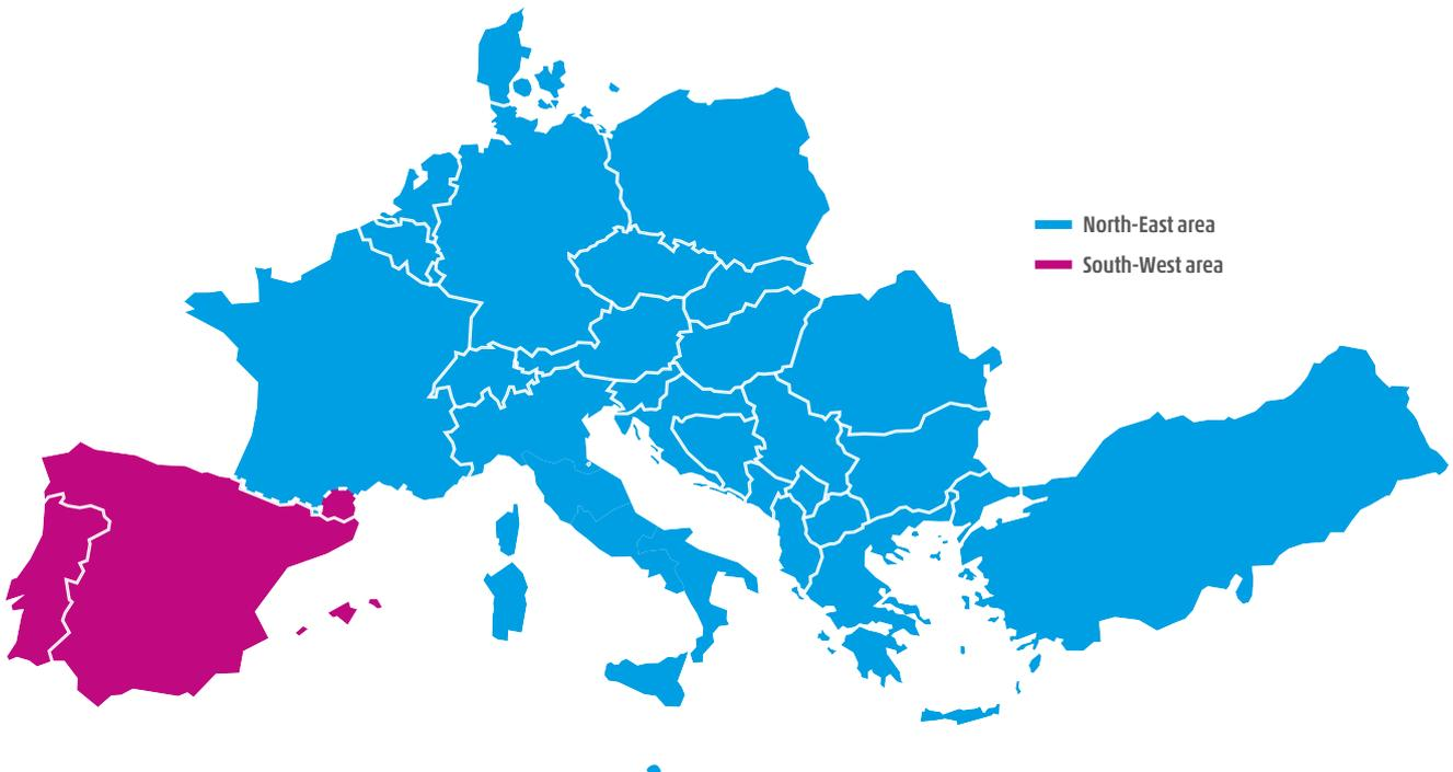
Figure 11: Resulting two synchronous areas after the system split.
