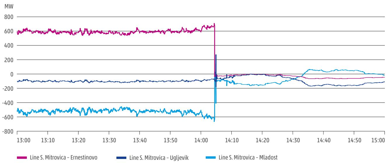
Figure A1-1: Power flows through the individual elements connected to busbars in SS Sremska Mitrovica 2
