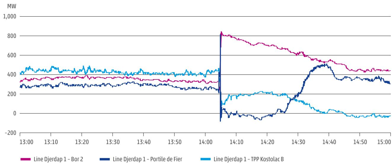
Figure A1-3: Power flows through the individual elements connected to busbars in SS Đerdap 1
