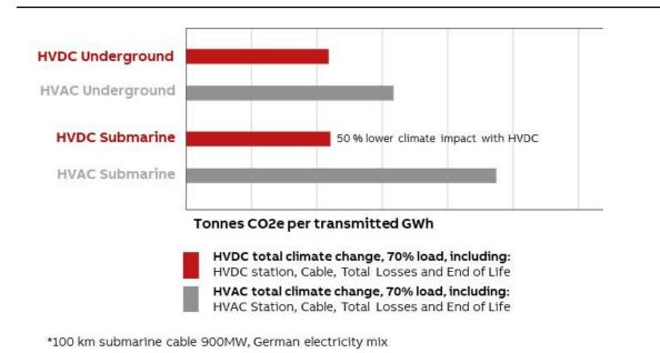
An HVDC link can reduce climate impact by half\* in terms of carbon footprint compared to an AC transmission link, thanks to lower transmission losses
